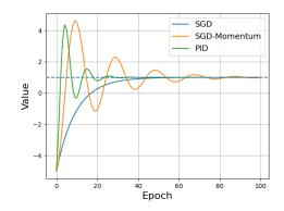
Fig. 2: Overshoot problem of SGD-Momentum and PID for quadratic function
